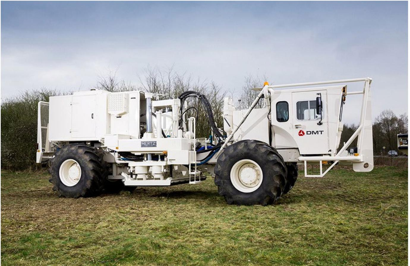
The Hemi 48 vibrator mounted on the M12 off-road chassis is an ideal seismic source unit if high quality results are needed from geophysical exploration.
