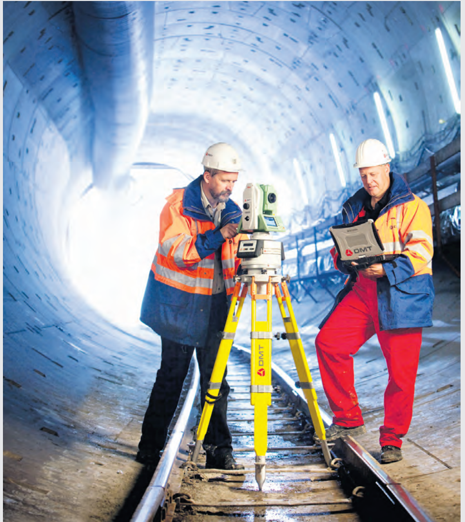
The Gyromat 5000: a surveying instrument for mine roadways delivering precision in tunnel engineering.
