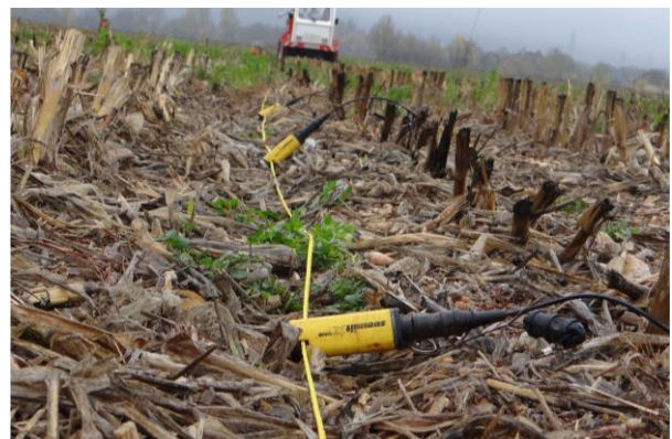
Field deployment for High-Resolution Vibro-Seis Survey
