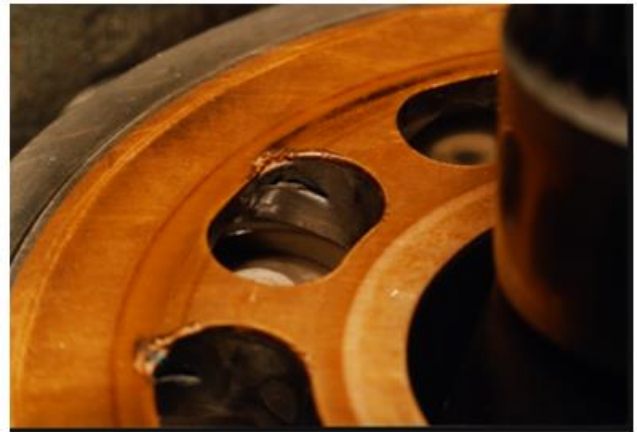
Cavitation damage at an axial piston pump
