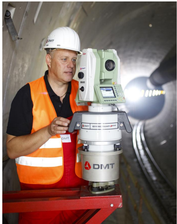
Orientation measurement with GYROMAT 3000
