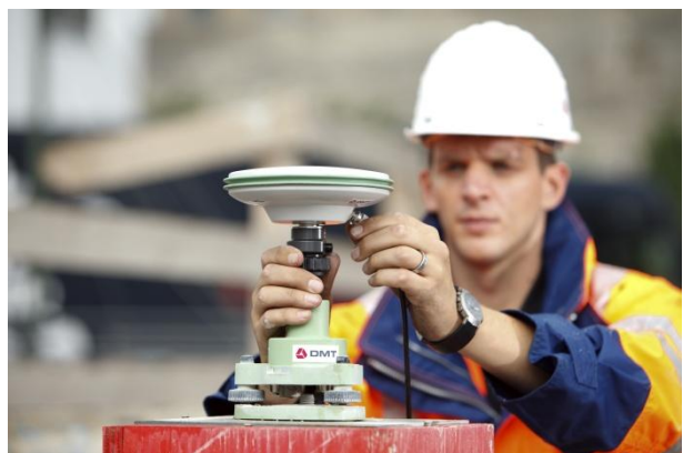
Static GPS measurement
