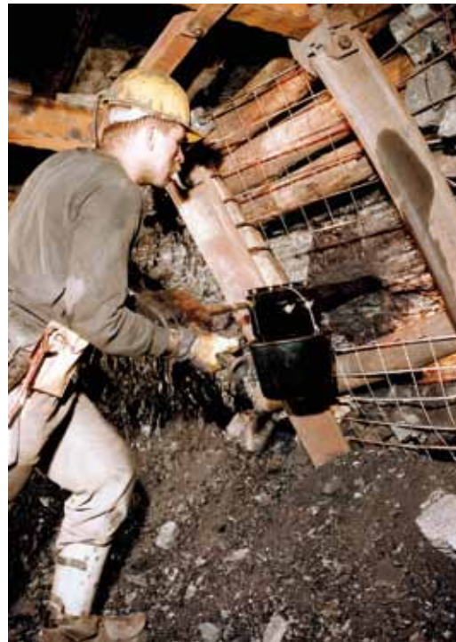
Test drilling – detection of rockburst hazards
