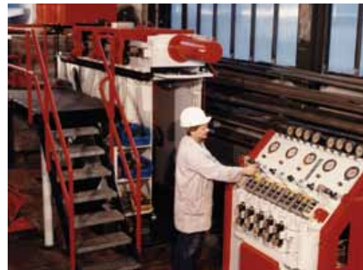
shear testing rig for installed rock bolts
