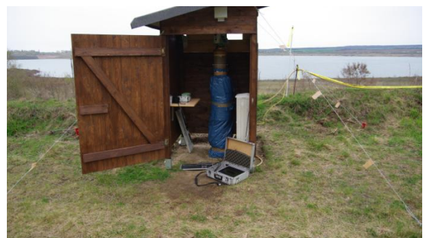
Total station in weatherproof housing
