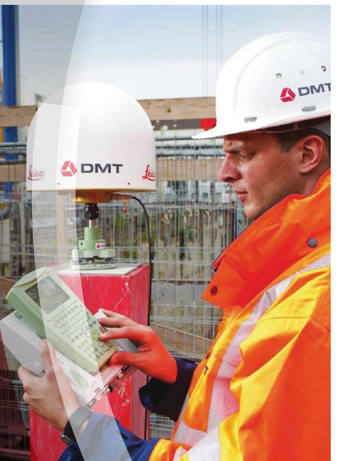
Monitoring with high precision GNSS equipment
