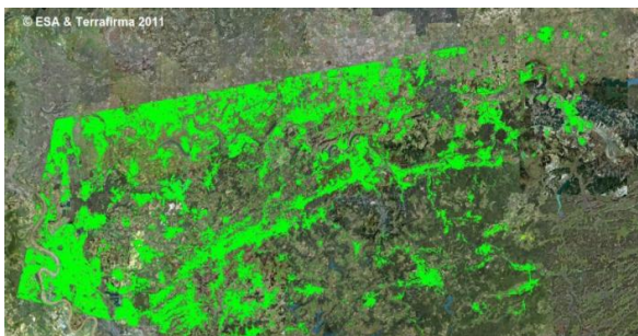
Large area PSI measurement result
