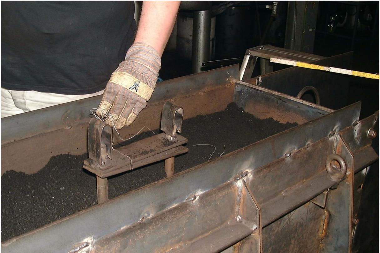
Figure 6: Facility of protection tubes to save the free space for monitoring probes positioning
