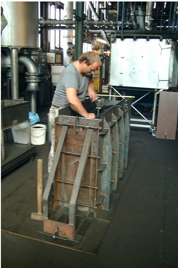
Figure 4: Stamp charging box for the movable wall oven
