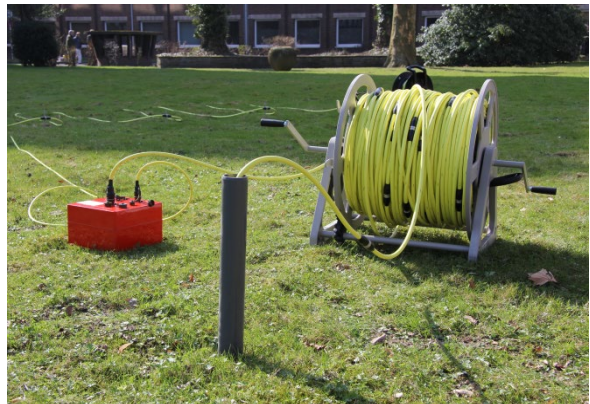
Borehole cable with decoder box
