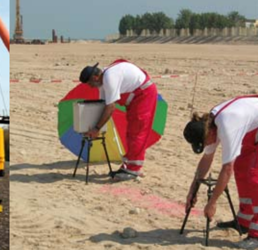
Gravity measurements during a construction site examination in Qatar
