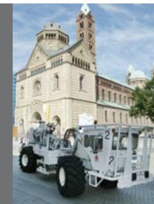
Deep vibroseismic examinations for a geothermy project in Speyer
