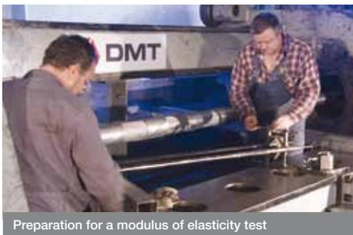
Preparation for a modulus of elasticity test
