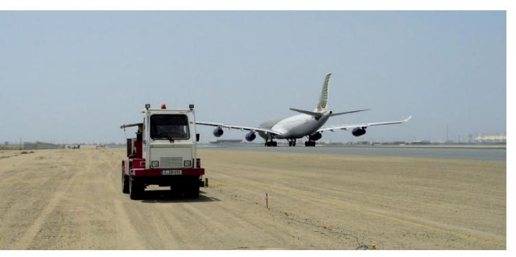
Seismic ground investigation in Jeddah
