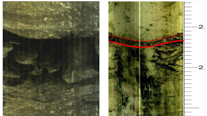
Borehole cable Borehole image of a shatter zones with decoder box
