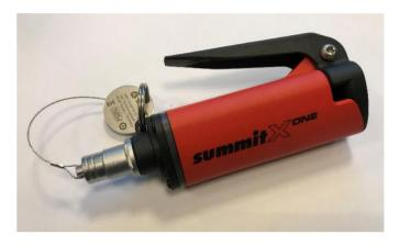
The Trigger Unit (TU) offers a very flexible alternative way of feeding the trigger signal into the SUMMIT X One seismic data acquisition system. Instead of connecting long trigger cables to the closest Data Collector Unit, the Trigger Unit can move with the source and connect to the SUMMIT X One Line cable at any place along the line using the same SNAP-ON Technology as the SUMMIT X One Remote Units.
