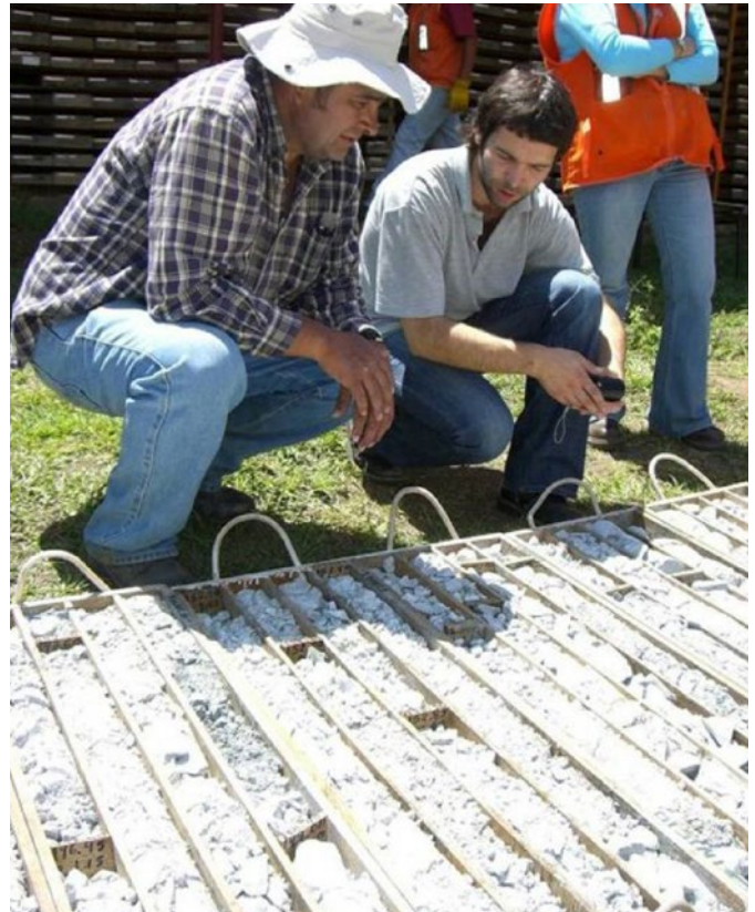
Heavily broken cores to scan and analyse
