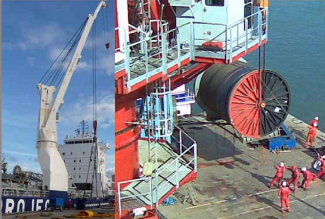
Heavy-lifting cranes on board
