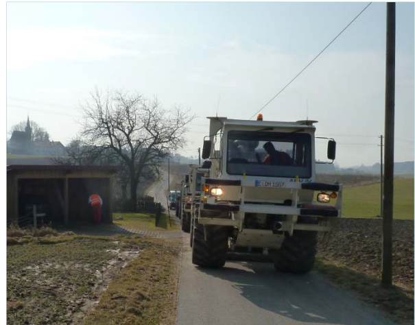
Vibroseis vehicle in the field during the WSP-survey in Traunreut
