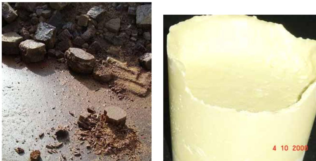
**Fig. 9: Stretford sulphur after autoclave (left) / Claus sulphur (right)**
