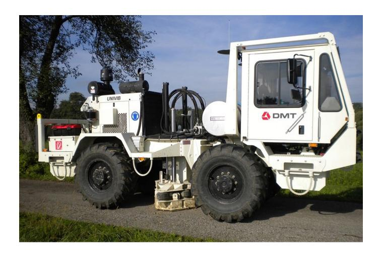
The UniVib™ Vibrator is a small vehicle which enables to operate in heavily urbanized areas or environmentally restricted areas. Due to it's small dimensions it is perfectly suited for small streets and can be applied without major field damages.
