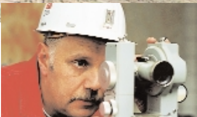
Uwe Kalz, DMT engineer, at work in Africa, carrying out a gyroscopic survey
